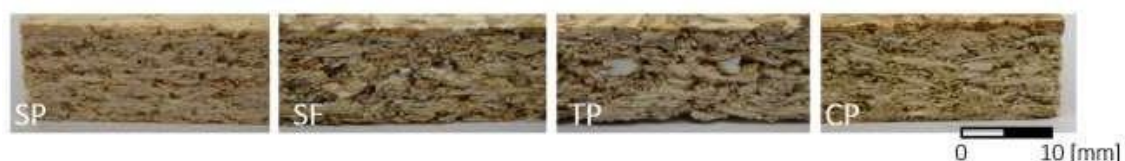
Figure 2. Cross sectional images of the produced particleboards, using spruce wood (SP), sunflower stalks (SF), topinambour stalks (TP), and cup-plant stalks (CP). (Petr et al. 2016)
